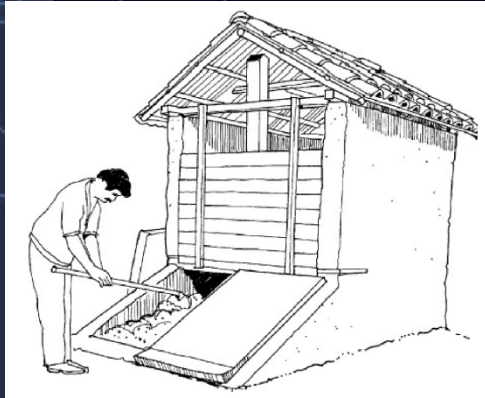
Double-vault dehydration toilet in Ecuador with inclined lids to increase the solar heating effect
